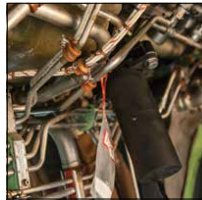
Digital Turning Tool installed on a gear box
